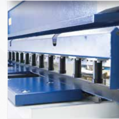
FINGER GUARD SWING-UP FEATURE FULL LENGTH
