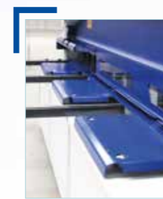
Standard Transfer table with roller balls and 1 Meter opening finger protection cover
