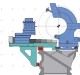
The anatomy of the V-series: four guides along which the slide, tailstock and steady rests move.
