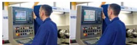
Swivelling control console, standard on all E-series machine tools: dazzling effect eliminated
