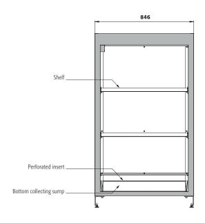
**Technical data** SP30.145.085.NE.WDFW External dimensions W x D x H 846 x 558 x 1451 mm Internal dimensions W x D x H 750 x 480 x 1135 mm Weight without interior equipment 219 kg Maximum load 600 kg Distributed load kg/m<sup>2</sup> 621 Capacity 165 litres (equals approx. 153 x 1-litre-bottles) Transport base entry height mm 95 Transport base entry width mm 680
