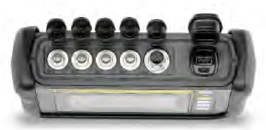
SCM-370-0-02 for 4 Parker analogue sensors with automatic sensor recognition and 2 auxiliary analogue sensors.
