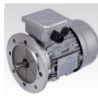
Standard Three-Phase Motors SM/I B5 230/400 V, 50 Hz 0,18 - 5,5 kW 750 - 3.000 /min Page 912
