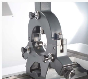
Steady rest with roller jaws Ø 12–150 mm
